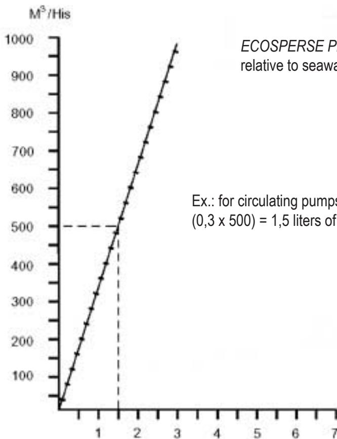
*ECOSPERSE PLUS* dosage in LITERS per HRS relative to seawater circulating pump. Capacity in M3/Hr.
