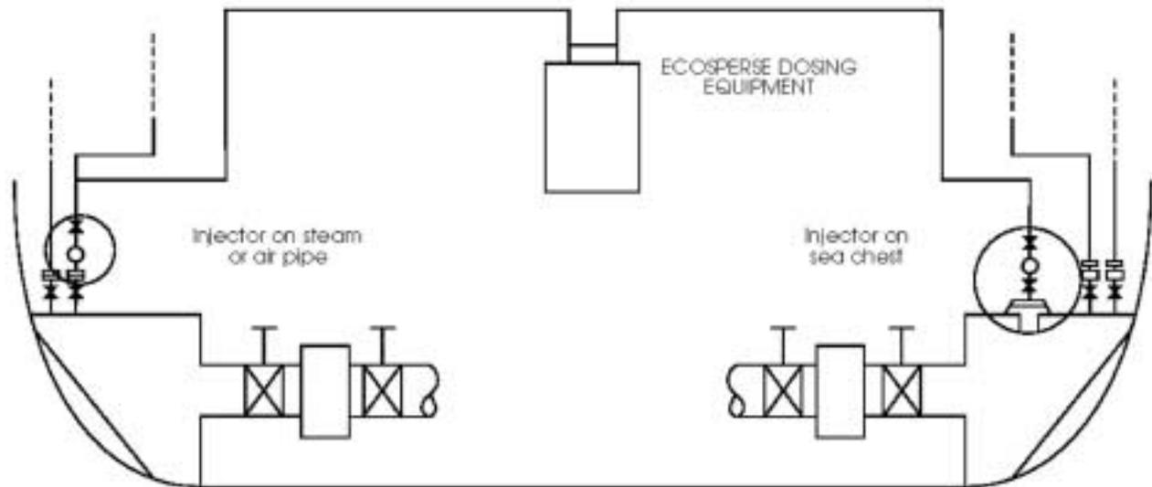
Typical installation of *ECOSPERSE PLUS* dosing equipment
